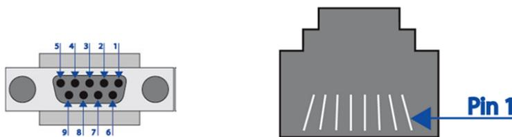
**Figure 50** DB-9 and RJ45 connector
